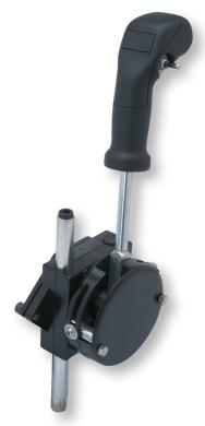
This lever, which is indicated for heavy duty applications and can be customize for specific applications, is used to command the hydraulic pump for the motion of the machine. Neutral, forward and reverse positions can be electrically signalled via micro-switch or via inductive sensor.
