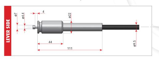
The end fittings are represented with the cable at mid stroke position
