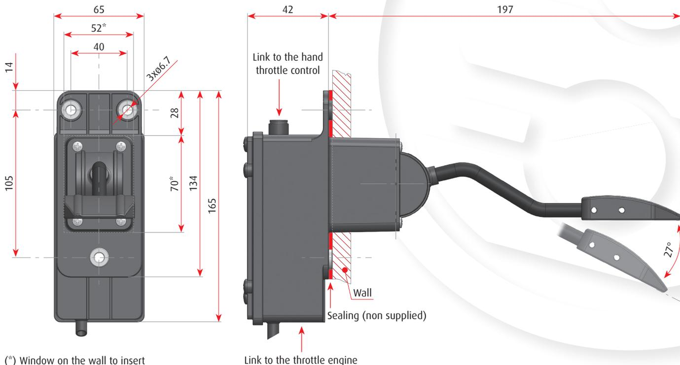
(\*) Window on the wall to insert the throttle pedal before the fixing
